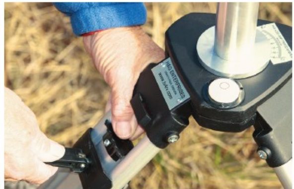
Below from left: Set the degrees of elevation and this custom aiming scope will enable you to check for obstructions in the line of sight. A solid aluminum machined mast is designed to fit a 2- or 1-5/8-inch bracket as well as supporting up to 35 pounds. The heavy-duty tripod has an infinite amount of adjustment for each leg, thus making the leveling process fast and easy.
