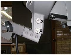
STEP 3 – Attach the LNB arm to the tilt plate using the hex bolts provided. Your model arm may be slightly different than the one shown. If not installed, put the RG-6 cable(s) into the LNB arm. If our Folding LNB Arm Kit has been installed, remove the two bolts, install the cable(s) and replace the bolts by installing them OVER the cable(s).
