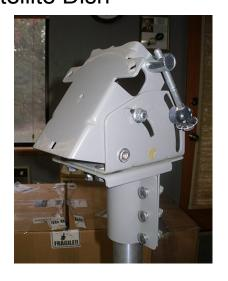
STEP 2 – Attach the Tilt Plate to the AZ-EL fixture using 3 stove bolts and either hex nuts or T knobs as provided.
